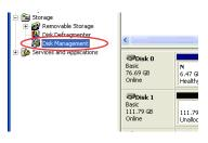
Locate the Disk that says it is "Unallocated" (check hard drive capacity to confirm it's the correct hard drive) and then right-click in the section that says "Unallocated" and select "New Partition".
